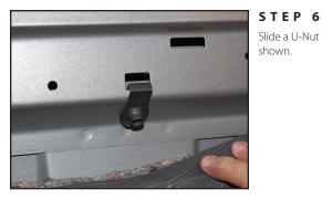
Slide a U-Nut in backwards through the rectangular hole as shown.
