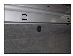
**STEP 3**If equipped, remove the snaps that hold the top of the carpet to the back of the cab.
