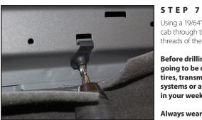
Using a 19/64" drill bit, drill a pilot hole into the back of the cab through the U-Nut. Use caution as to not damage the threads of the U-Nut or hit the outer cab wall.
